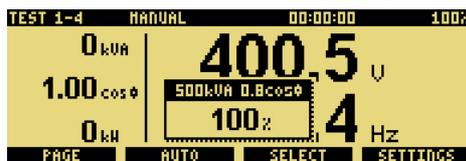
Pressing the **SELECT** key changes between load control in %, kW or kVA and power factor. If a resistive-only load bank is used, then the selection will be % and kW only.
