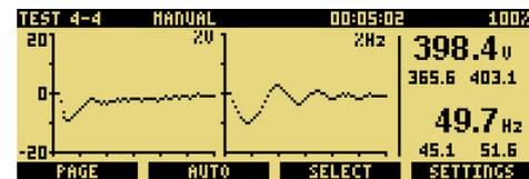
The voltage and frequency graphs display the first 6 seconds of the last load change, as a percentage of the supply voltage and frequency rating.
