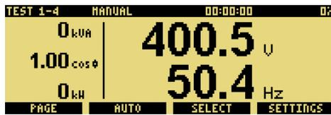
You can select and apply load on any of the four **TEST** pages in the same way.
