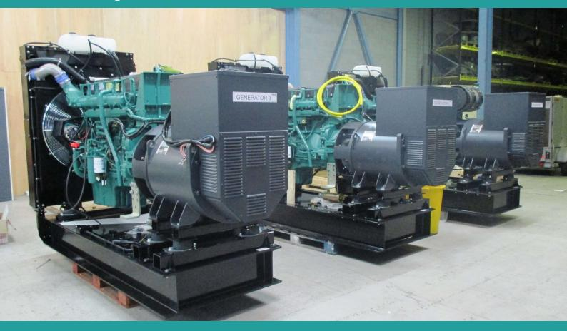
With the upgrade of any back-up power system old parts are often no longer fit for purpose and new components are usually inevitable. We replaced an existing day fuel tank and installed 3 day new base fuel tanks as well as introducing a new fuel polishing unit to the existing fuel bulk tank to keep the fuel clean and avoid contamination.
